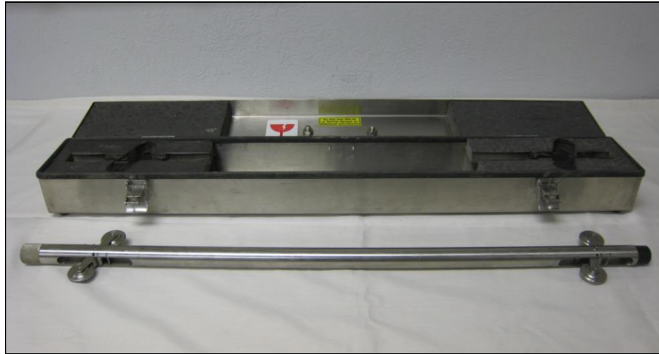
Figure 3-30: The Slope Indicator inclinometer probe and its container.
