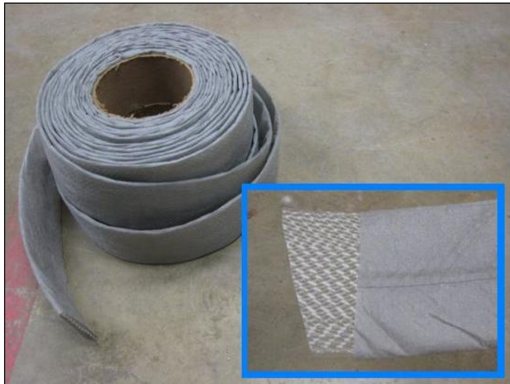
Figure 3-10: Wick drain material used in this study.
