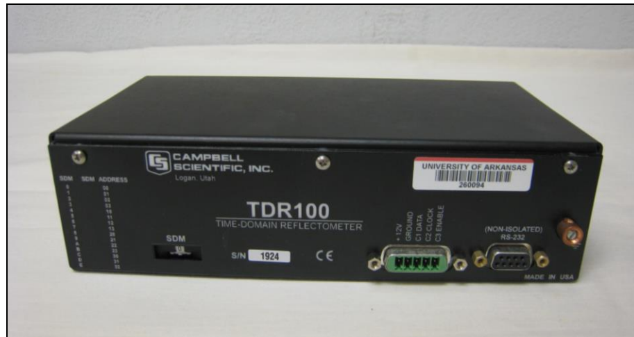
Figure 3-15: A Campbell Scientific TDR100 used in the research.
