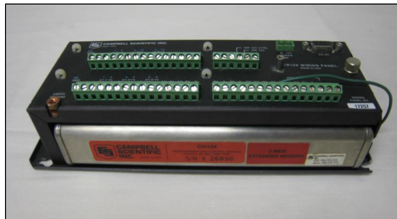
Figure 3-12: A datalogger CR10X used in the research.
