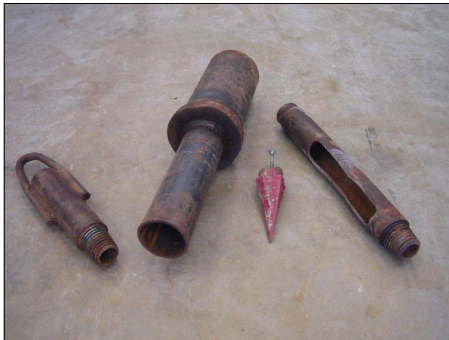
Figure 3-42: From left to right, pulling-head, drive head, steel drive point, and slotted drive tube used in the wick drain installation.
