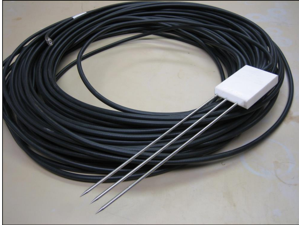
Figure 3-21: A CS610 moisture probe used in the study.
