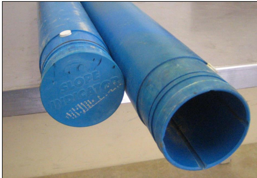
Figure 3-32: Quick Connect (70 mm) inclinometer casings used in the study.
