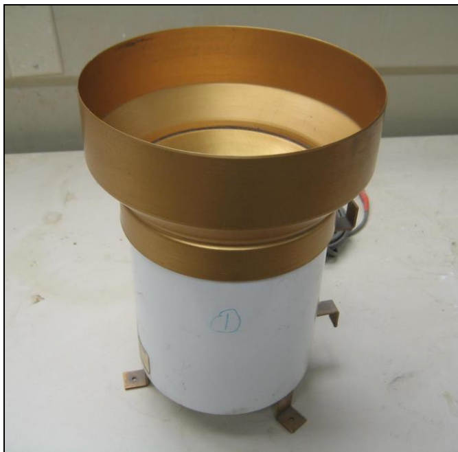
Figure 3-24: Model rain gauge used in the study.
