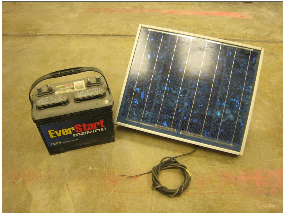
Figure 3-25: Solar panel and 12-V battery used to supply power to the TDR system.
