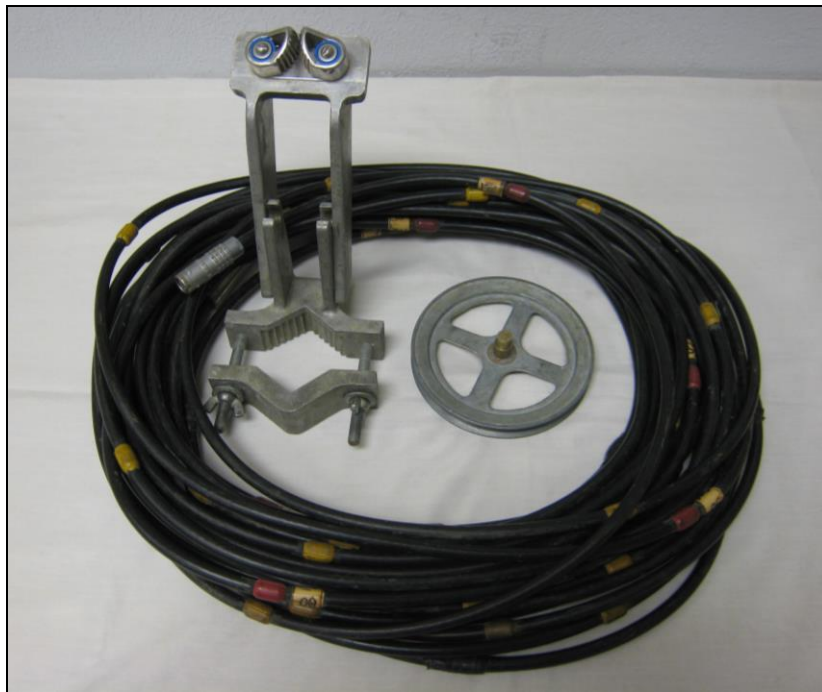
Figure 3-32: The control cable and the pulley assembly for inclinometer system.
