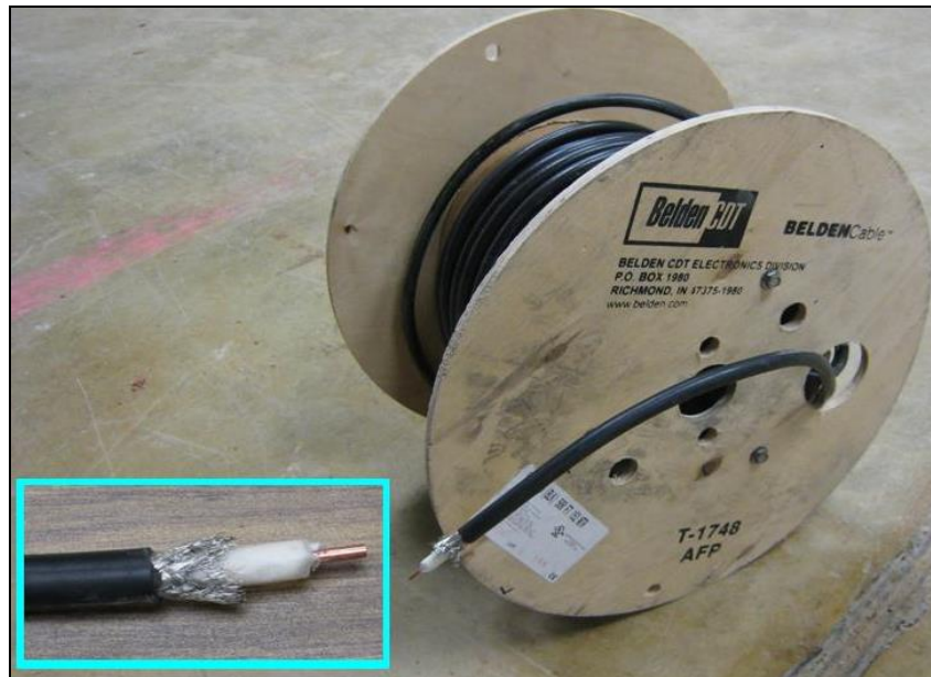
Figure 3-19: The RG8 TDR coaxial cable used in the research.
