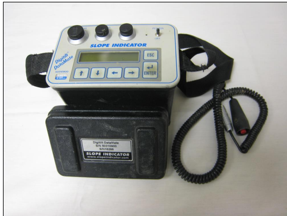
Figure 3-31: The Digitilt DataMate® readout unit (After Slope Indicator).
