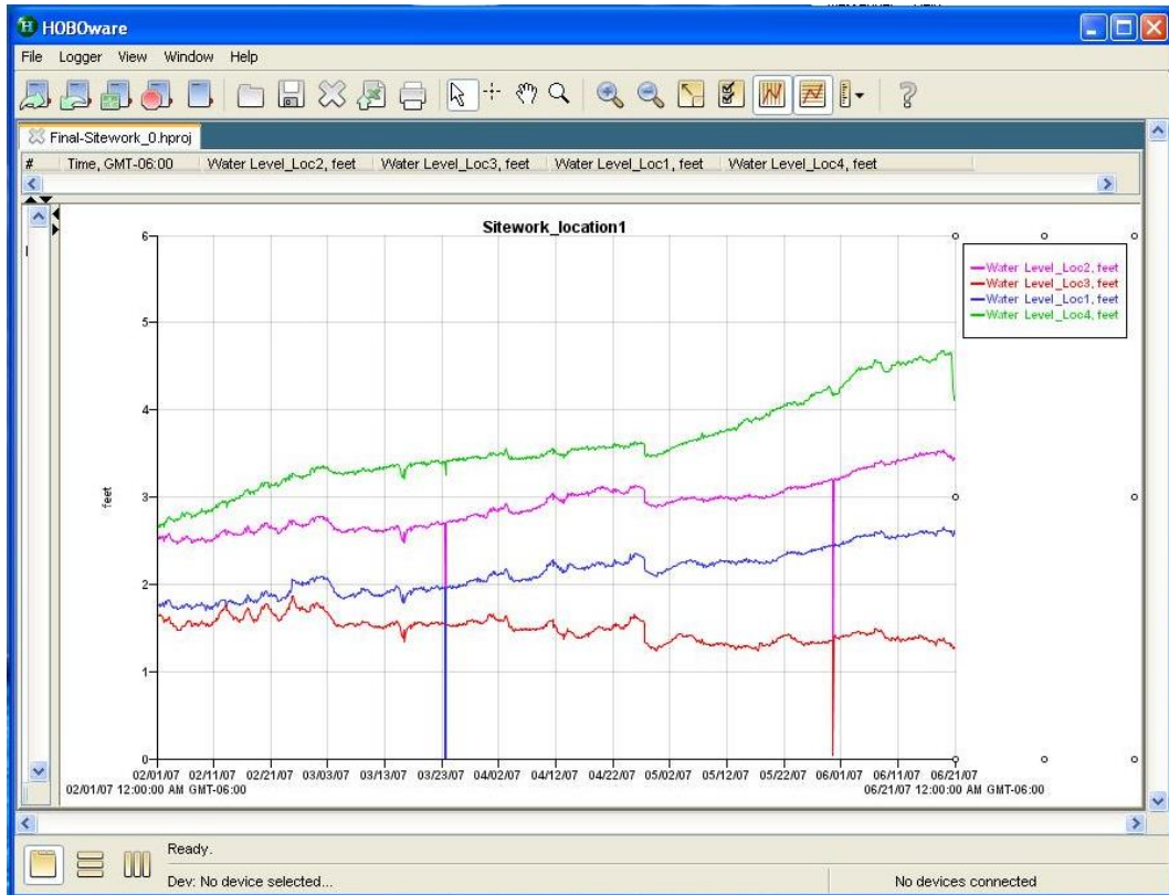
Figure 4-40: Ground water table profile at all locations.
